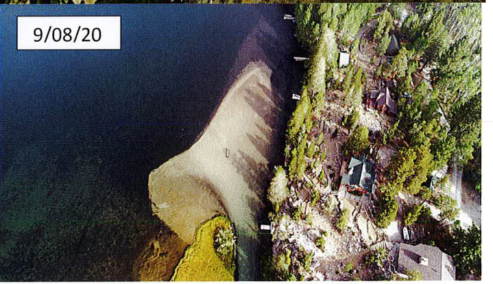
Aerial views of the enlarging sand plume due to sedimentation in the Rush Creek channel at the confluence with Silver Lake
