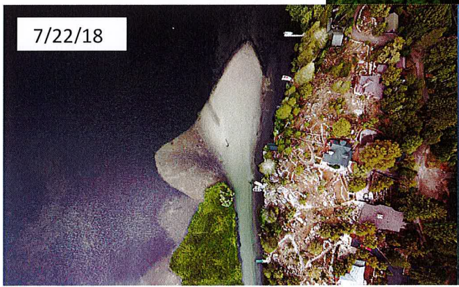
Aerial views of the enlarging sand plume due to sedimentation in the Rush Creek channel at the confluence with Silver Lake
