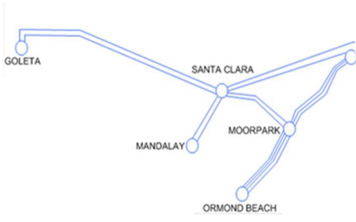
A-Bank Substations in Moorpark Sub-Area
